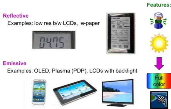
Figure 3: Display technologies: Reflective (top) with low power consumption and sunlight readability but mostly monochrome visualization. Emissive displays (bottom) with multimedia have high power consumption and are suitable for indoor use.
